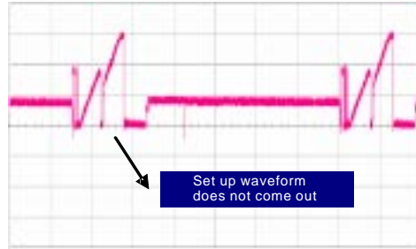
<Fig. 3 When the Set_Down FET is damaged>
